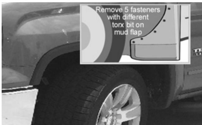
Make sure the front tire has been turned outward for easy installation. **FOR MODELS WITH FACTORY MUDFLAP:** Remove 5 mud flap fasteners with T-30, T-15 torx bit & screw driver. Save the upper two fasteners for re-install in step 7.
