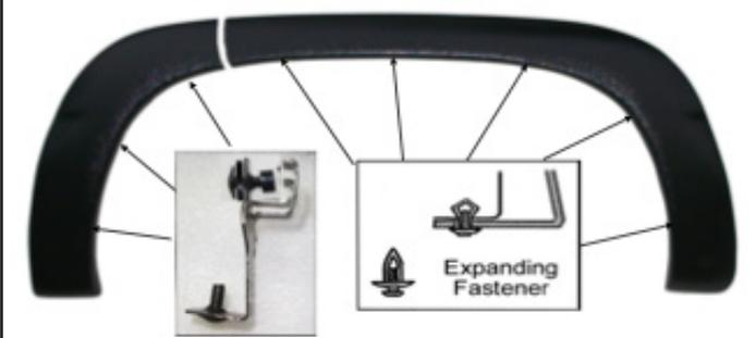
Place the flare on the vehicle. Apply 5 Plastic Expanding Fasteners into the mounting slots in the flare and secure it to the vehicle as shown. Mount 3 sets of Y-Clips with Flange Type-B screws, plastic ring and caps on the door part of the flare. Secure it to the vehicle.
