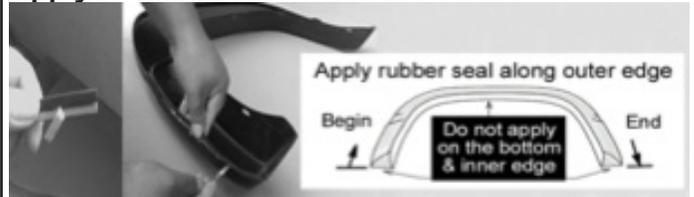
Remove about 1 inch of tape liner from rubber seal and apply it to the flare. Start at one end of the flare along the edge that comes in contact with the body panel. Apply pressure on the tape to ensure adhesion, and trim excess rubber seal at the end. To avoid bulge you may cut a notch in the edge of the rubber seal at the inward angle curve. Cut a V out for the outward angle curve.
