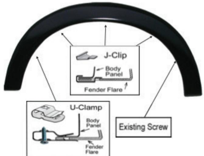
Place the flare on the vehicle. Apply 3 J-Clips into the mounting slots in the flare and secure it to the vehicle, 1 U-Clamp secures into the hole with flat head screws as shown. Fasten the existing factory screws into the original location that were previously removed.
