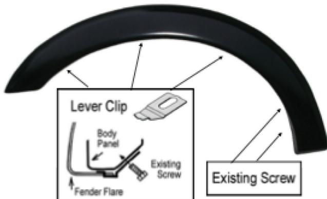
Place the flare on the vehicle. Apply 3 Lever Clips, secure it to the hole with existing screws as shown. Fasten the existing factory 2 screws into the original location that were previously removed.
