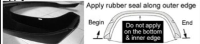
Apply rubber seal to the flare. Start at one end of the flare along the edge that comes in contact with the body panel. Apply pressure on the tape to ensure adhesion, and trim excess rubber seal at the end. To avoid buldge, you may cut a notch in the edge of the rubber seal at the inward angle curve, cut a V out for the outward angle curve.
