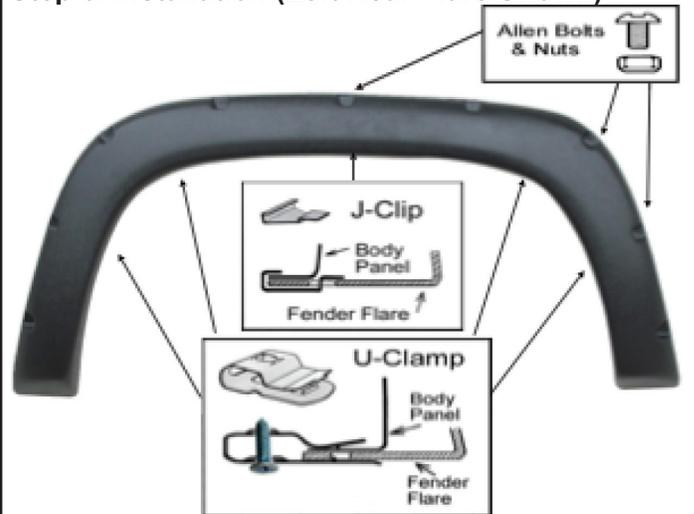
Use torx bit to tighten allen bolt & put firmly on every pocket of the fender flares. **DO NOT OVER TIGHTEN!** Place the flare on the vehicle. Apply 1 J-Clip into the mounting slots in the flare and secure it to the vehicle. Use 4 U-Clamps and secure it into the hole with hex screws as shown.
