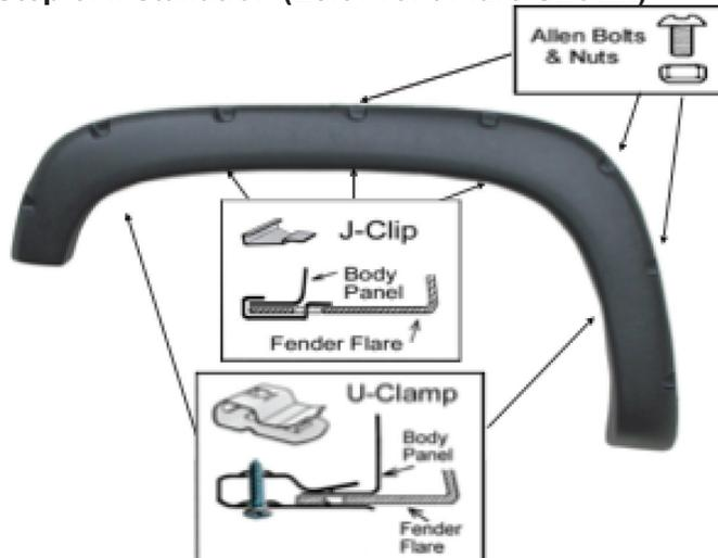
Use torx bit to tighten allen bolt & put firmly on every pocket of the fender flares. **DO NOT OVER TIGHTEN!** Place the flare on the vehicle. Apply 3 J-Clips into the mounting slots in the flare and secure it to the vehicle. Use 2 U-Clamps and secure it into the hole with hex screws as shown.
