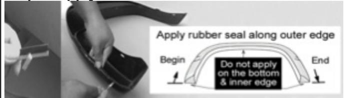
Remove about 1 inch of tape liner from rubber seal and apply it to the flare. Start at one end of the flare along the edge that comes in contact with the body panel. Apply pressure on the tape to ensure adhesion, and trim excess rubber seal at the end.
