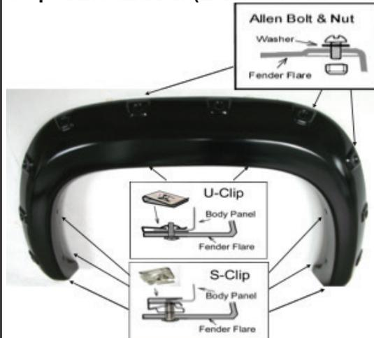
Use tory bit to tighen allen bolt & nut firmly on every pocket of the fender flares. **DO NOT OVER TIGHTEN!** Hold the flare in position on the vehicle, use a grease pencil to mark eight hole locations. Apply 2 U-Clips over two top marks, align with holes in flare. Apply 6 S-Clips over six lower marks, align with holes in flare. Adjust the clips in position, use 2 flange screws and 6 truss machine screws to secure it as shown.
