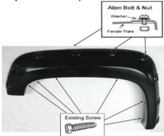
Use tory bit to tighten allen bolt & nut firmly on every pocket of the fender flares. **DO NOT OVER TIGHTEN!** Remove 6 existing screws from the fasteners on the vehicle. Place the flare on the vehicle with best position. Reinstall the existing factory screws into the original location that were previously removed. Do not tighten the screws fully until the flares are aligned and extrusive against the body.
