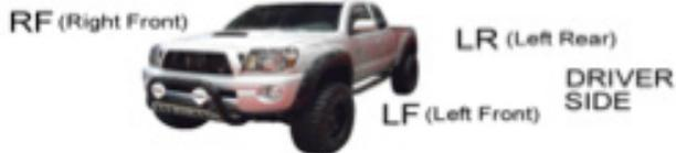
Prefit both driver side and passenger side fender flares to the vehicle before painting or installation. You may remove any moldings, strips or existing flares from the vehicle for fitting or installation. You can cut the fender flare to fit any body side molding.
