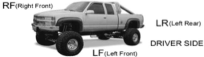
Prefit both driver side and passenger side fender flares to the vehicle before painting or installation. You may remove any moldings, strips or existing flares from the vehicle for fitting or installation. You can cut the fender flare to fit any body side molding.
