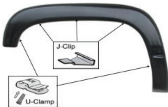
Place the flare on the vehicle. Apply 3 J-Clips into the mounting slots in the flare and secure it to the vehicle. Use 2 U-Clamps and secure it into the hole with hex screws as shown.
