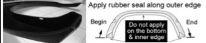
Apply rubber seal to the flare. Start at one end of the flare along the edge that comes in contact with the body panel. Apply pressure on the tape to ensure adhesion, and trim excess rubber seal at the end. To avoid buldge, you may cut a notch in the edge of the rubber seal at the inward angle curve, cut a V out for the outward angle curve.
