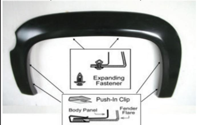
Place the flare on the vehicle. Apply 2 Plastic Expanding Fasteners into the mounting slots in the flare and secure it to the vehicle as shown. Apply 4 Push-In Clips into the mounting slot in the flare and secure it to the vehicle as shown.
