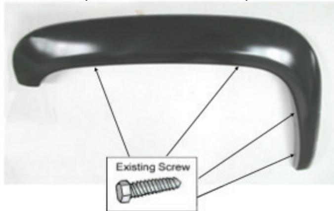
Remove 4 existing screws from the fasteners on the vehicle. Place the flare on the vehicle. Reinstall the existing factory screws into the original location that were previously removed. Do not tighten the screws fully until the flares are aligned and extrusive against the body.
