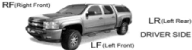
Pre-fit both driver side and passenger side fender flares to the vehicle before painting or installation. You may remove any moldings, strips or existing flares from the vehicle for fitting or installation. You can cut the fender flare to fit any body side molding.
