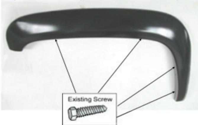
Remove 4 existing screws from the fasteners on the vehicle. Place the flare on the vehicle. Reinstall the existing factory screws into the original location that were previously removed. Do not tighten the screws fully until the flare are aligned and extrusive against the body.
