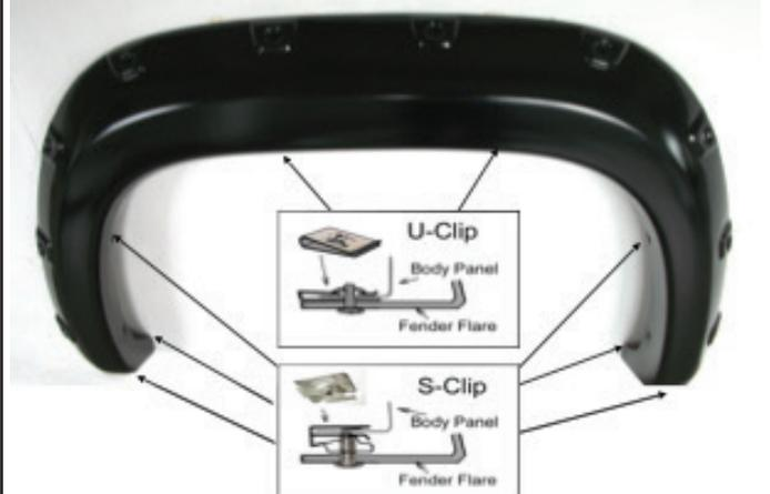
Hold the flare in position on the vehicle, use a grease pencil to mark eight hole locations. Apply 2 U-Clips over two top marks, align with holes in flare. Apply 6 S-Clip over six lower marks, align with holes in flare. Adjust the clips in position, use 2 flange screws and 6 truss machine screws to secure it as shown.
