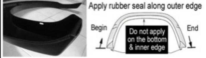
Apply rubber seal to the flare. Start at one end of the flare along the edge that comes in contact with the body panel. Apply pressure on the tape to ensure adhesion, and trim excess rubber seal at the end. To avoid bulge you may cut a notch in the edge of rubber seal at the inward angle curve, cut a V out for the outward angle curve.
