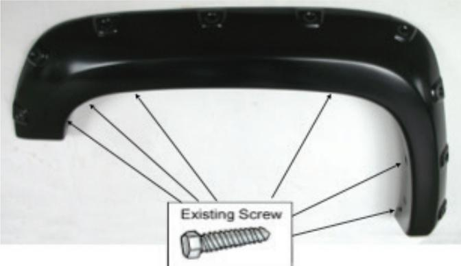
Remove 6 existing screws from the fasteners on the vehicle. Place the flare on the vehicle. Reinstall the existing factory screws into the original location that were previously removed. Do not tighten the screws fully until the flares are aligned and extrusive against the body.
