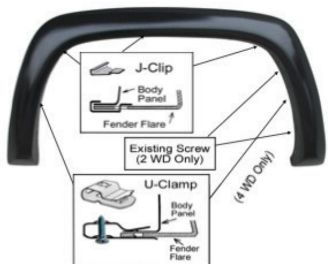
Place the flare on the vehicle. Apply 3 J-Clips into the mounting slots in the flare and secure it to the vehicle. Use 2 U-Clamps and secure into the hole with flat head screw as shown. Fasten the existing factory screws into the original location that were previously removed for 2 WD.
