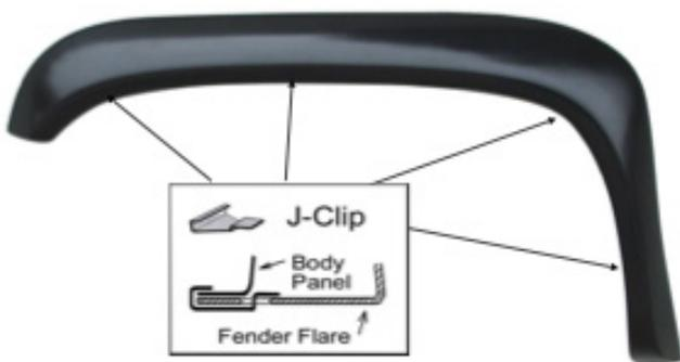
Place the flare on the vehicle. Apply 4 J-Clips into the mounting slot in the flare and secure it to the vehicle as shown.
