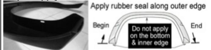
Apply rubber seal to the flare. Start at one end of the flare along the edge that comes in contact with the body panel. Apply pressure on the tape to ensure adhesion, and trim excess rubber seal at the end. To avoid bulge you may cut a notch in the edge of rubber seal at the inward angle curve, cut a V out for the outward angle curve.
