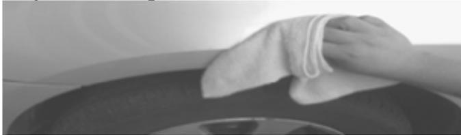
Wash and wipe dry the areas of contact on the vehicle body. Clean the surface and inside edge of the fender flare where the rubber seal is to be attached.
