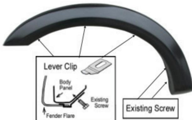
Place the flare on the vehicle. Apply 3 J-Clips into the mounting slot in the flare and secure it to the vehicle as shown. Fasten the existing factory 2 screws into the original location that were previously removed.
