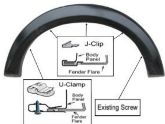
Place the flare on the vehicle. Apply 3 J-Clips into the mounting slots in the flare and secure it to the vehicle. Use 1 U-Clamp and secure it into the hole with flat head screw as shown. Fasten the existing factory screws into the original location that were previously removed.
