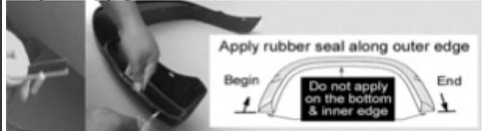
Remove about 1 inch tape liner from rubber seal and apply it on the flare. Start one end of the flare along the edge that comes in contact with the body panel. Apply pressure on the tape to ensure adhesion, and trim excess rubber seal at the end.
