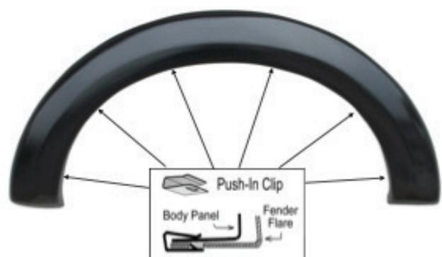
Place the flare on the vehicle. Apply 6 Push-In Clips into the mounting slots in the flare and secure it to the vehicle as shown.
