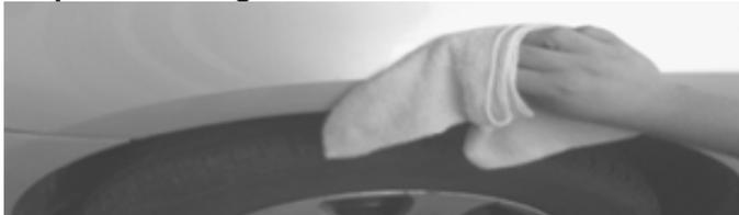
Wash and wipe dry the areas of contact on the vehicle body. Clean the surface and inside edge of the fender flare where the rubber seal is to be attached.
