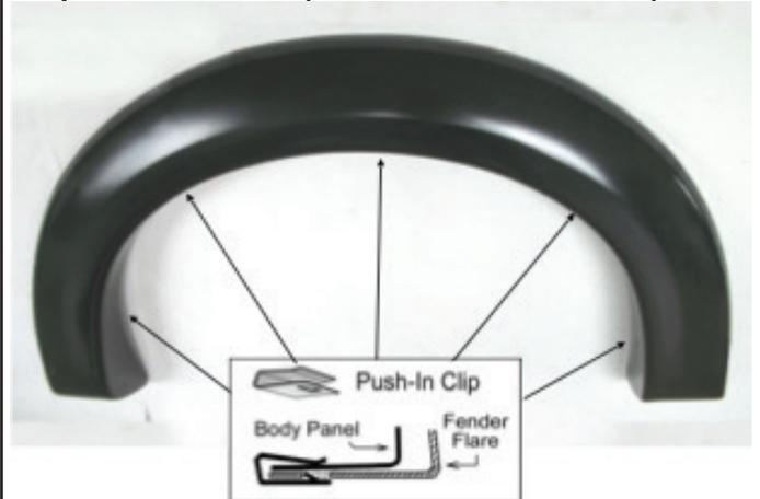
Place the flare on the vehicle. Apply 5 Push-In Clips into the mounting slot in the flares and secure it to the vehicle as shown.
