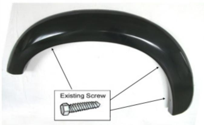
Place the flare on the vehicle. Fasten the existing factory screws into the original location that were previously removed.
