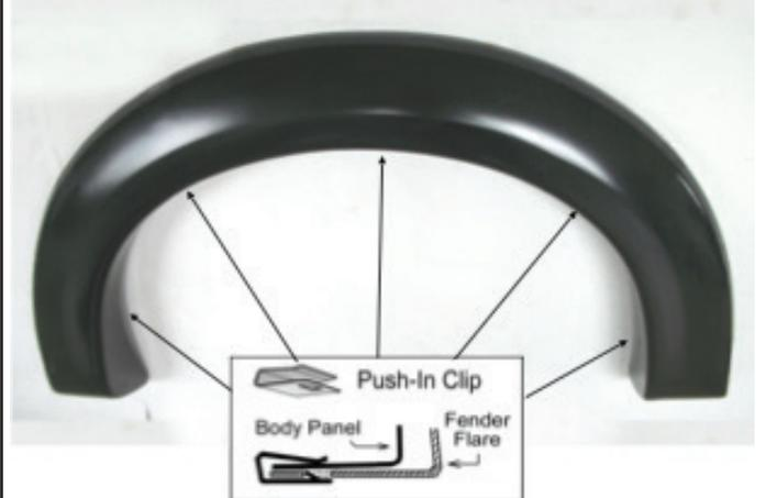
Place the flare on the vehicle. Apply 5 Push-In Clips into the mounting slot in the flares and secure it to the vehicle as shown.
