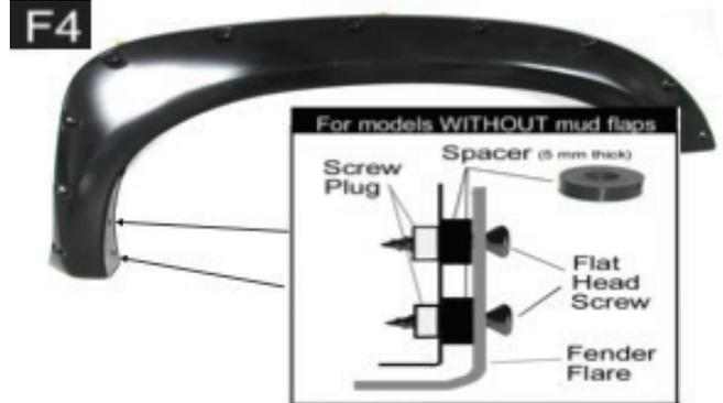
Insert the supplied spacer (5mm thick) in between vehicle body & flare, apply 2 flat head screws to secure the flare to the body as shown.
