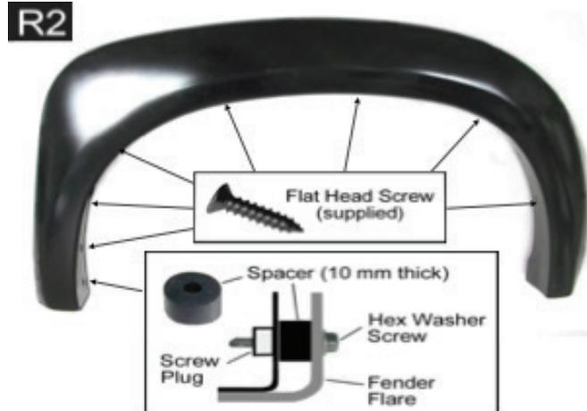
Fasten 7 flat head screws into the location, shown as center. Insert the supplied spacer (10mm) in between vehicle body & flare, apply 1 hex washer screw to secure the flare to the body.
