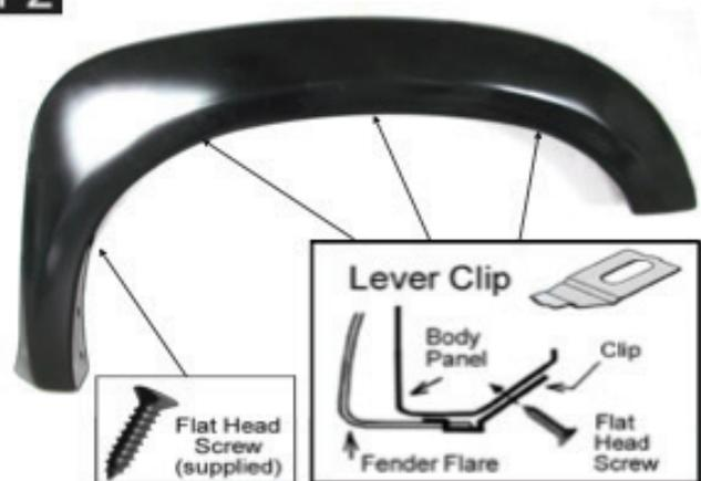
Apply 3 Lever Clip into the mountain slot in flare and secure it to the vehicle with flat head screw, shown as right. Fasten 1 flat head screw into the location, shown as left.
